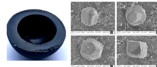
UHMWPE/MWCNT Acetabular cup and the wear debris generated from it after 5 million cycle of simulator test against stainless steel femoral head
